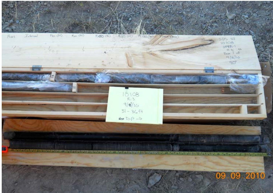
Photograph 9: UPRR-1, 31.0 to 36.0 feet bgs. Claystone of the Graneros Shale formation. Sample in top core barrel from 31.0 to 32.8 feet and in bottom of core barrel below 32.8 feet.
