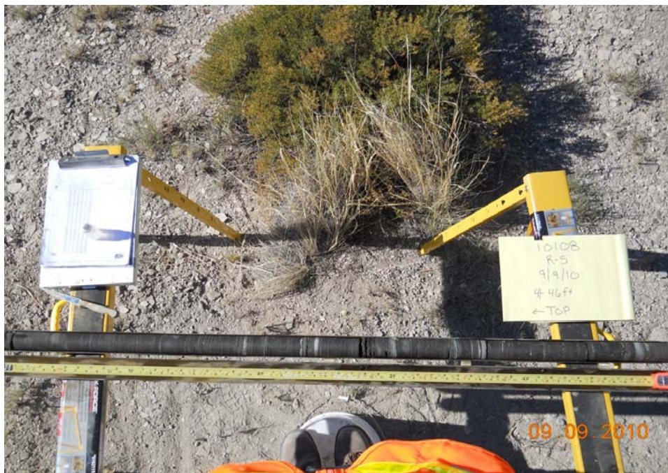
Photograph 10: UPRR-1, 41.0 to 46.0 feet bgs. Claystone with sandstone lenses.
