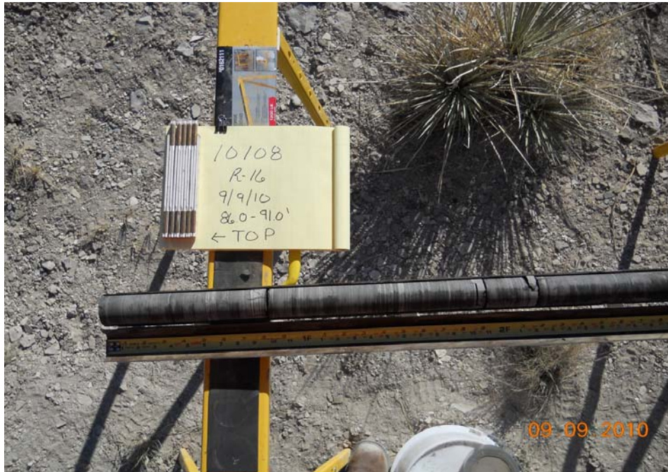
Photograph 11: UPRR-1, 86.0 to 88.9 feet bgs. Interbedded claystone and sandstone of the Graneros Shale formation.
