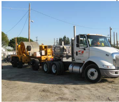
Figure 13-1 Reel Carrier and Tractor
