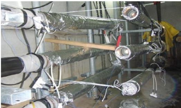
Figure 13-3 Preparation of Cable Ends
